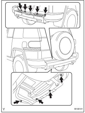
(b) Remove the 7 bolts and the 2 screws.
